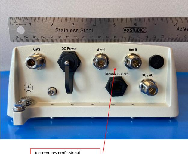
Unit requires professional installation to ensure the proper antenna is employed.
