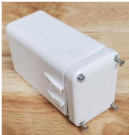
Figure 2-5: Removing the Battery Cover Screws
