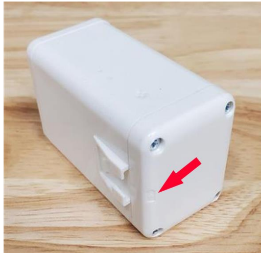
Figure 2-8: Proper Replacement Orientation of the Battery Cover
