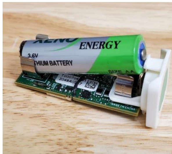
Figure 2-3: Battery Polarity Orientation
