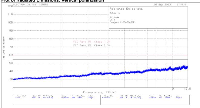
Test Sample: FCC Part 15.247 Report #: t29e23a302\_DTS Seal/Seal Ex Release 2 FCC ID:2ALEPT0007705
