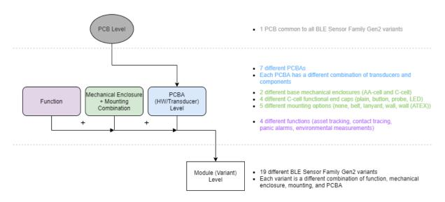
Figure 1-1: Gen2 BLE Sensor Family Groupings and Hierarchy
