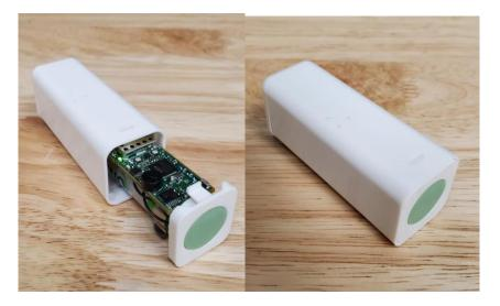
Figure 2-7: Replacing the PCBA and End-Cap
