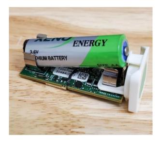
**Figure 2-6: Battery Polarity Orientation**
