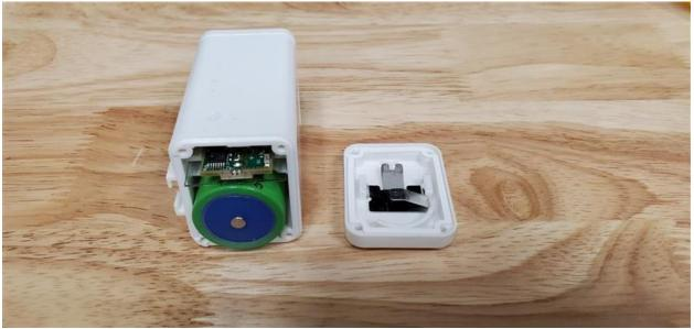
Figure 2-9: Battery Polarity Markers and Insertion
