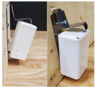
Figure 2-3: Attaching the Sensor to the Mounting Bracket
