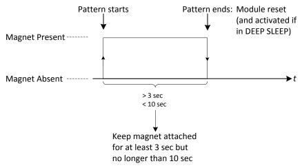
Figure 2-1: The C-Cell Sensor Variant Magnetic Activation Pattern
