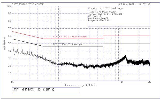
Test Sample: AC Outlet FCC Part 15.247 Report #: t29e20a162\_Outlet-DTS\_FCC FCC ID: 2ALEPT0006623 (902 – 928 MHz) Release 1
