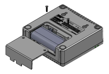
**Figure 6: Battery Installation**
