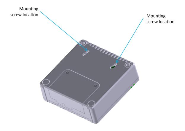
**Figure 3: Kona Micro PoE Gateway Mounting Screw Locations**
