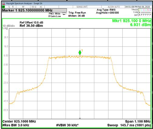
Screen Capture from Spectrum Analyzer: 500 KHz Channel High (DTS Mode)
