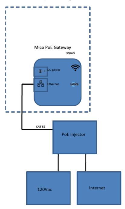
Micro PoE Gateway test setup for emission tests
