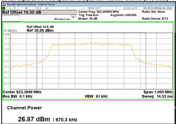
Screen Captures from the spectrum analyzer: 500 KHz MID Channel (DTS MOD)
