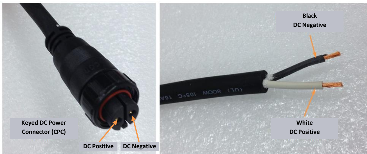
Figure 6: Direct DC Power CPC Connector Connection Polarity
