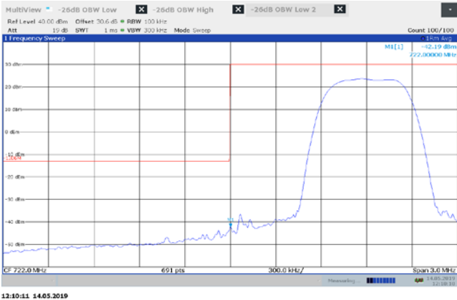
Figure 8.2-8: Lower band edge for single carrier
