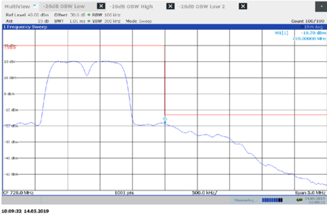
Figure 8.2-11: Upper band edge for two carrier
