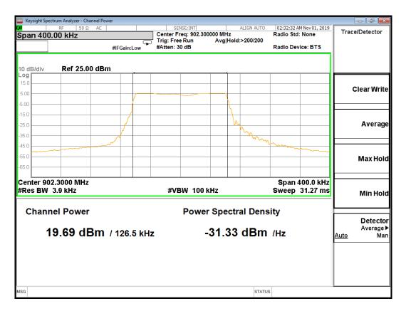
Screen Captures from the spectrum analyzer: 125 KHz MID Channel (Hybrid Mode)
