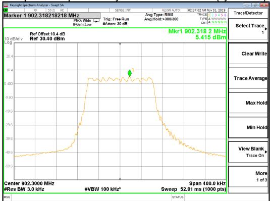
Screen Capture from Spectrum Analyzer: 125 KHz Channel MID (Hybrid Mode)
