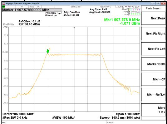
Screen Capture from Spectrum Analyzer: 500 KHz Channel High (DTS Mode)
