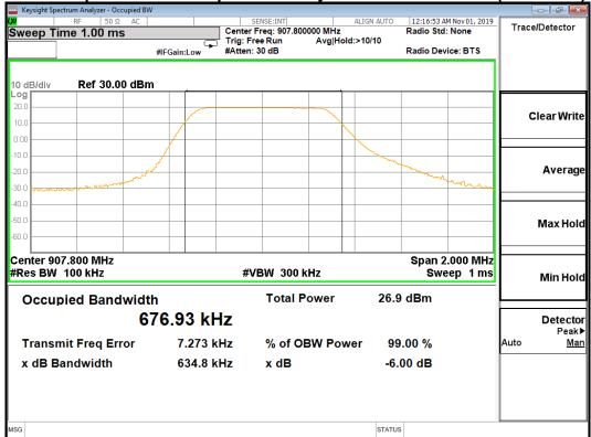
Screen captures from the spectrum analyzer 500 KHz Channel (DTS Mode)
