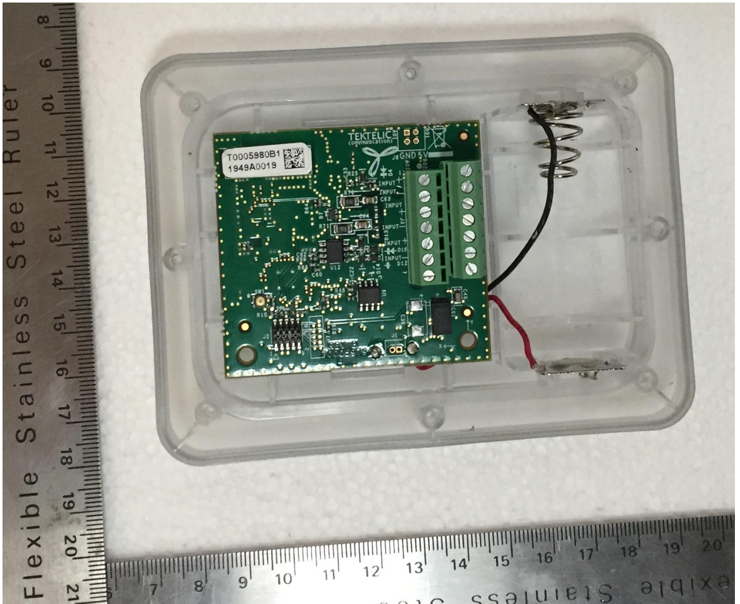
Top Cover with PCB and Battery Holder No Battery (T0005986 Variant)
