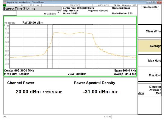
Screen Captures from the spectrum analyzer: 125 KHz MID Channel (Hybrid Mode)
