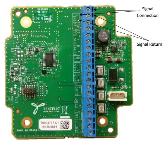
Figure 2-2: The Industrial Sensor external connector signals.
