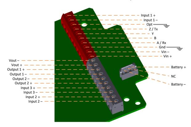
Figure 1-2: The Industrial Sensor interface layout (terminal block and battery connector pinout).
