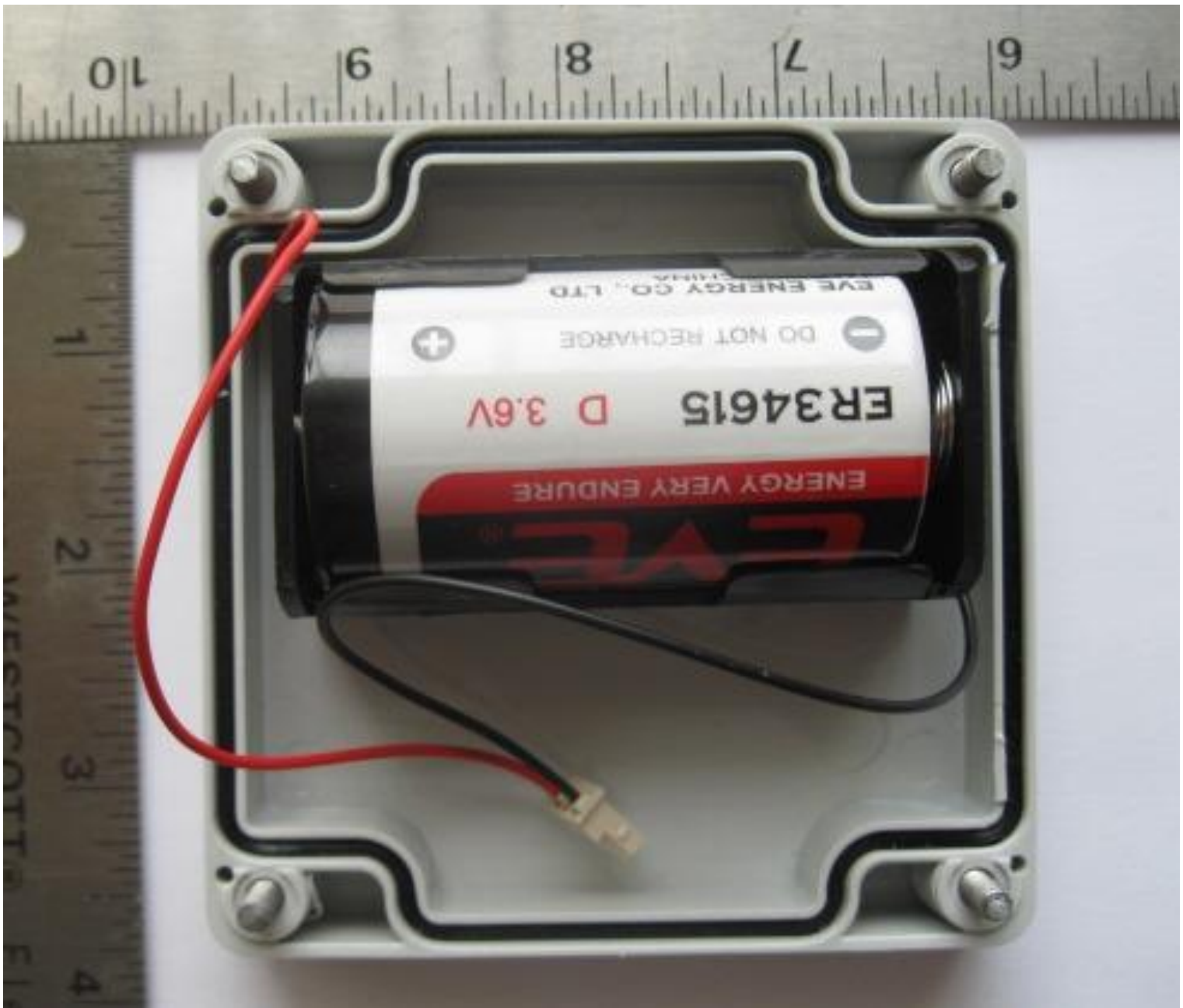
Top Cover battery holder with battery
