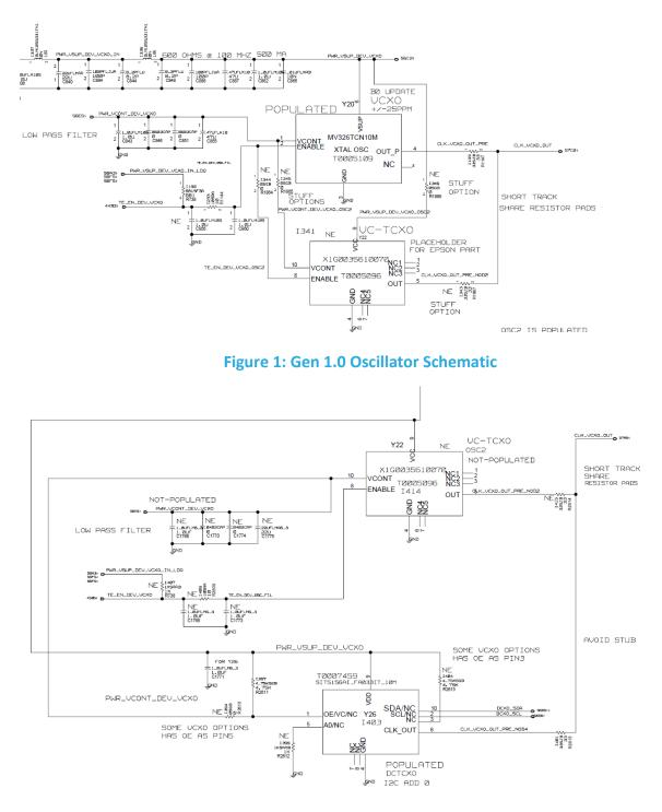
Figure 2: Gen 1.5 Oscillator Schematic
