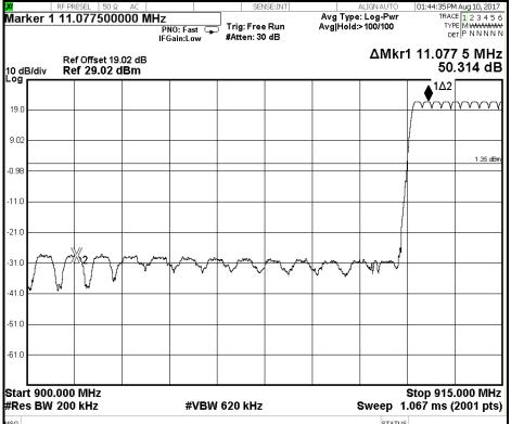
Screen Capture from the spectrum analyzer: Upper Band Edge (Hopping)
