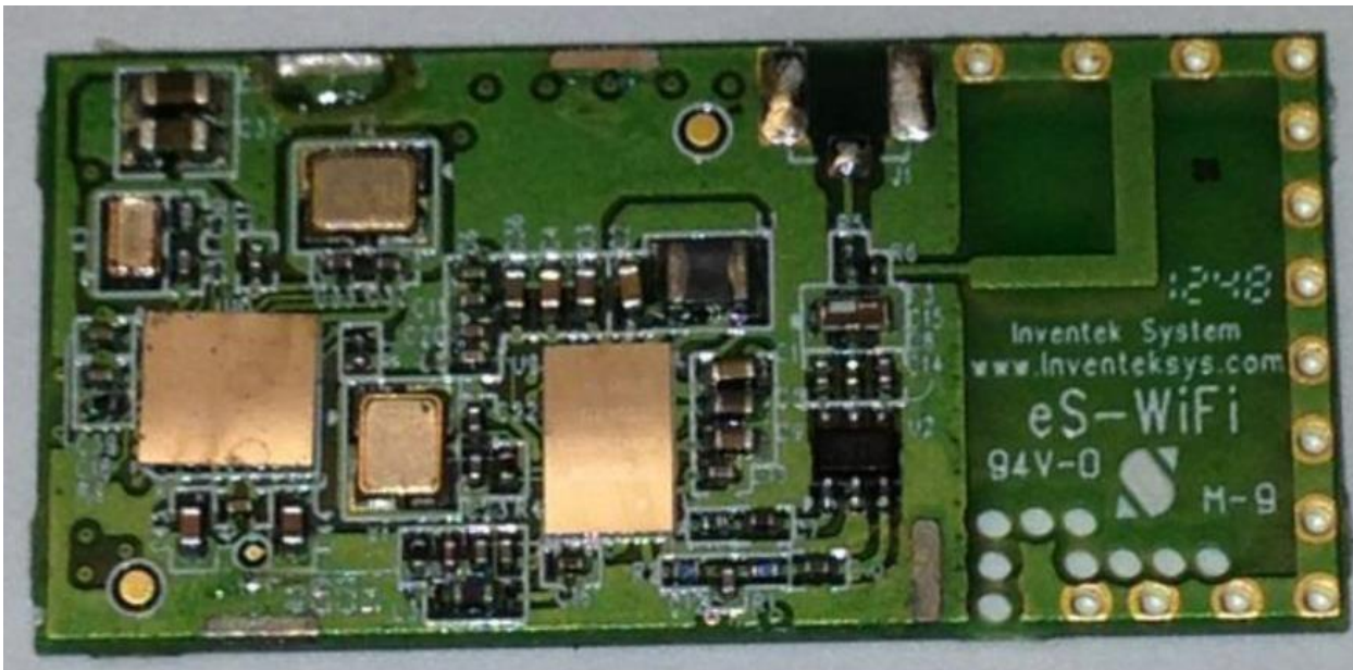
WiFi module (FCC ID: O7P-362, IC: 10147A-362) component side without shield
