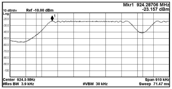
Screen Capture from spectrum analyzer: Antenna 0, 2 Carrier, 925.1 MHz
