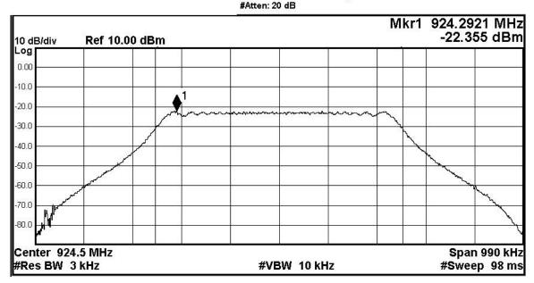
Screen Capture from spectrum analyzer: Antenna 0, 1 Carrier, 925.1 MHz
