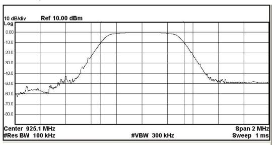
Occupied Bandwidth Total Power 6.49 dBm 656.90 kHz
