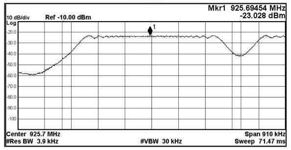
Screen Capture from spectrum analyzer: Antenna 1, 2 Carrier, 926.3 MHz
