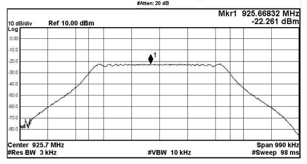
Screen Capture from spectrum analyzer: Antenna 1, 1 Carrier, 926.3 MHz
