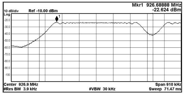
Screen Capture from spectrum analyzer: Antenna 1, 2 Carrier, 927.5 MHz
