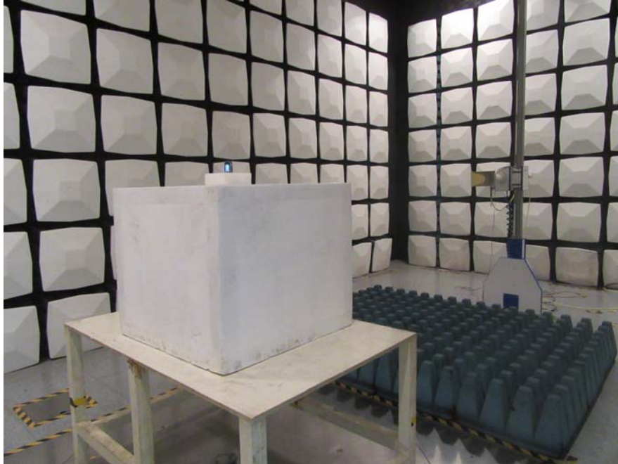
Radiated Emission View (Above 1GHz)
