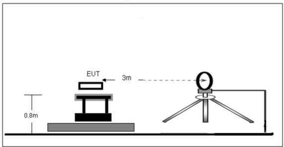
(B) Radiated Emission Test-Up Frequency 30MHz~1GHz
