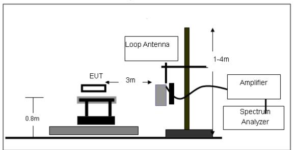
(B) Radiated Emission Test-Up Frequency 30MHz~1GHz
