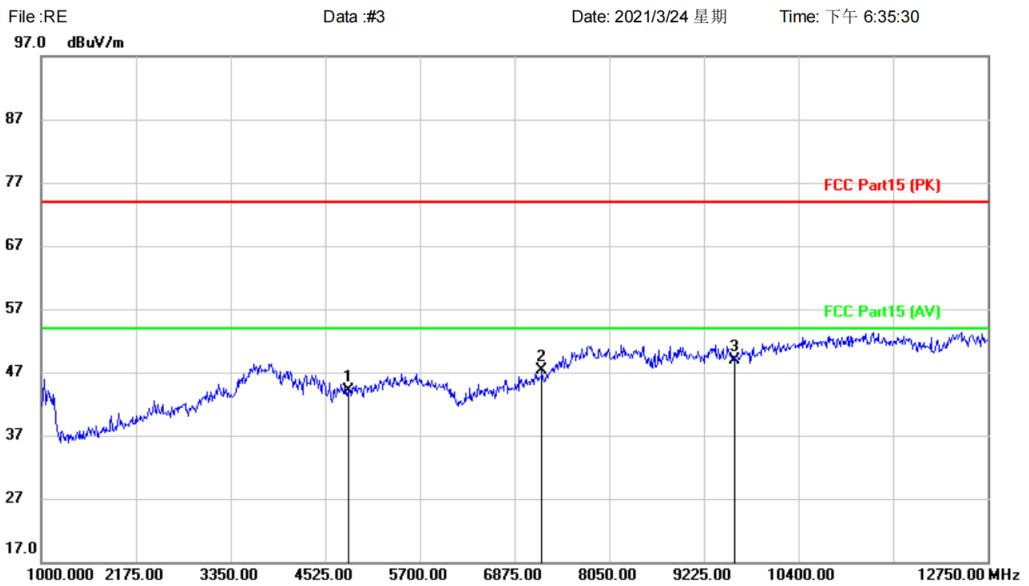
Site                              Polarization: **Horizontal**                      Temperature:
