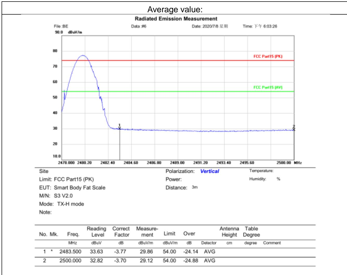
**Radiated Emission Measurement**
