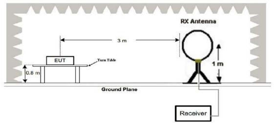
(2) Radiated Emission Test-Up Frequency 30MHz~1GHz
