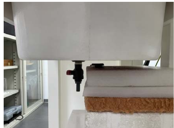
Fig.6 Front side of EUT (Rubber) to flat phantom
