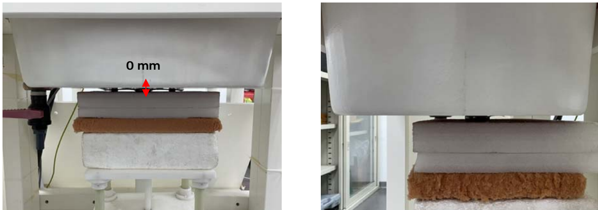
Fig.4 Back side of EUT (Rubber) to flat phantom
