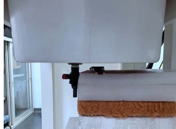
Fig.5 Front side of EUT (Matel) to flat phantom
