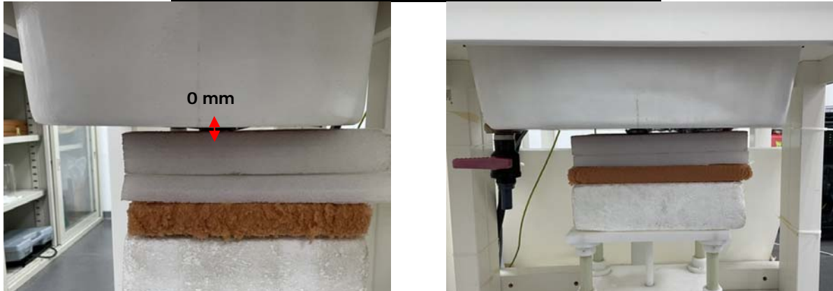
Fig.3 Back side of EUT (Metal) to flat phantom
