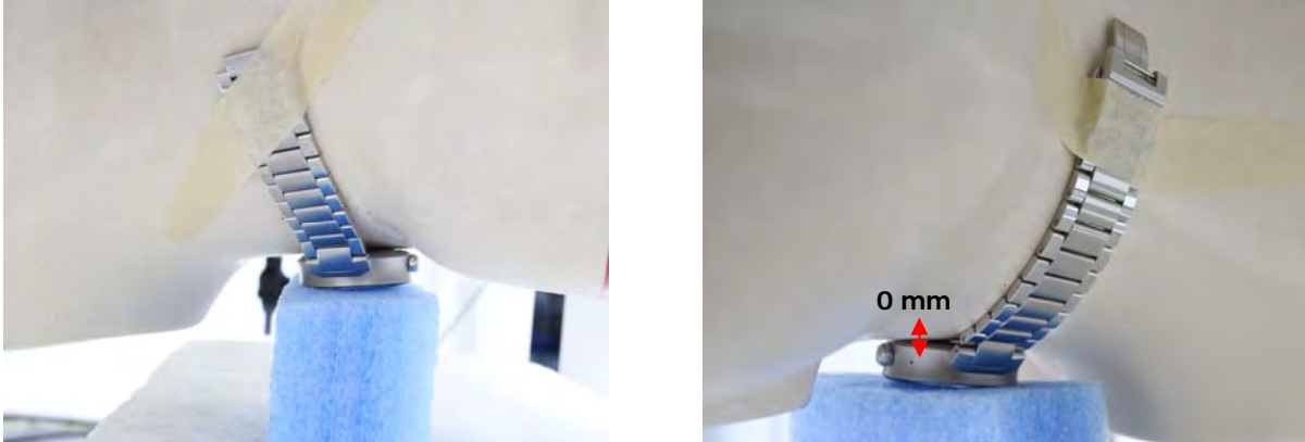
Fig.3 EUT backside touch against the neck phantom area
