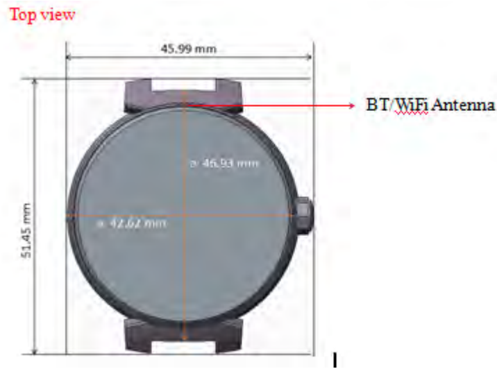
Fig.6 Antenna location (Front view)
