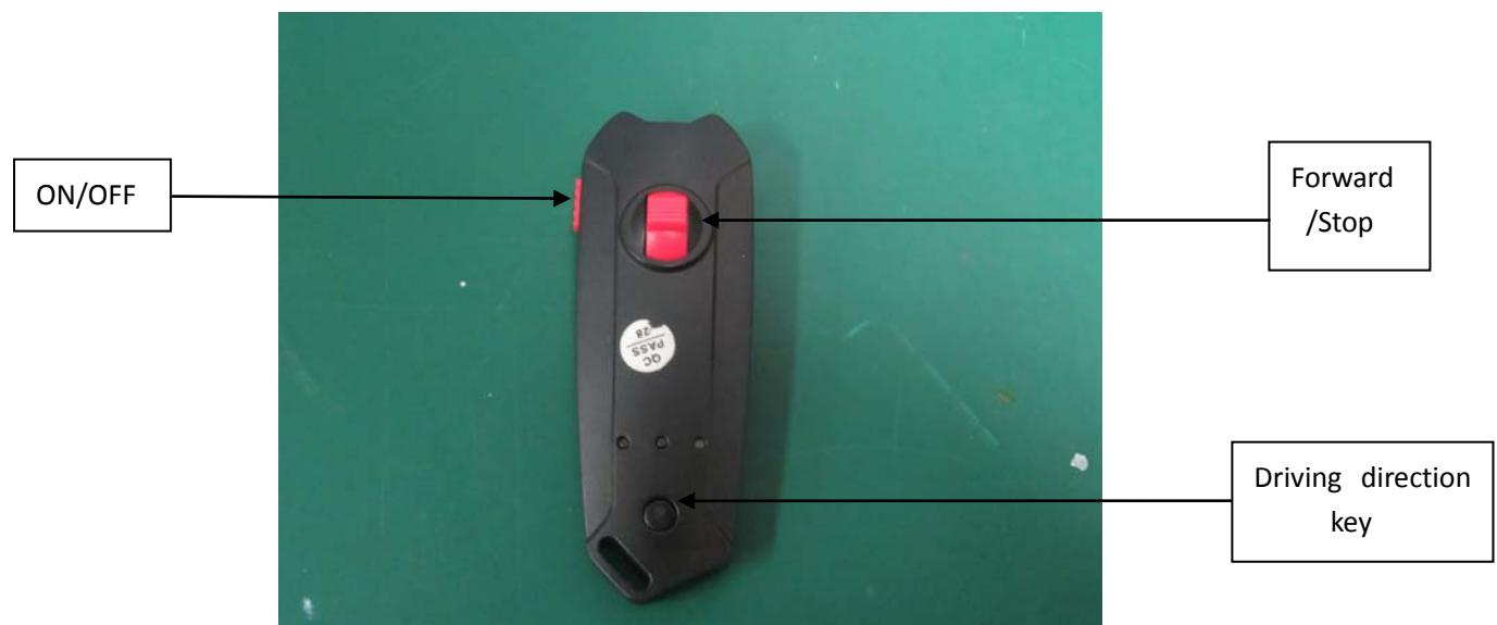
Open the remote control power switch, remote control buzzer sound (small fish no beep). Dial the lever, then remote control led lights flash. If not, please follow the fault instructions;
