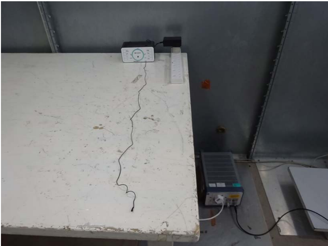
Measurement of Conducted Emission Test Set Up
