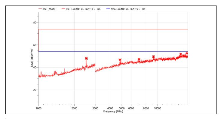
Temperature: **EUT:** SmartSet Clock Radio 24.5℃ M/N.: ER100301 **Humidity:** 55%RH **Power Rating:** Mode: 3-DH5 2441MHz AC 120V/60Hz **Test Engineer: Test Time:** 2023-08-03 **Berny**
