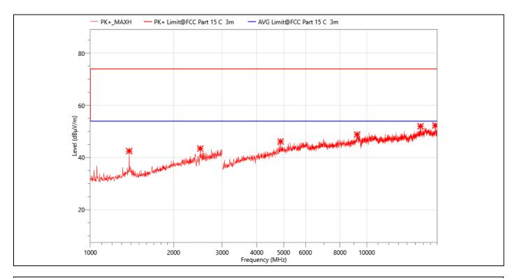
**EUT:** SmartSet Clock Radio **Temperature:** 24.5℃ M/N.: ER100301 **Humidity:** 55%RH **Power Rating:** Mode: 3-DH5 2402MHz AC 120V/60Hz **Test Engineer: Test Time:** 2023-08-03 **Berny**
