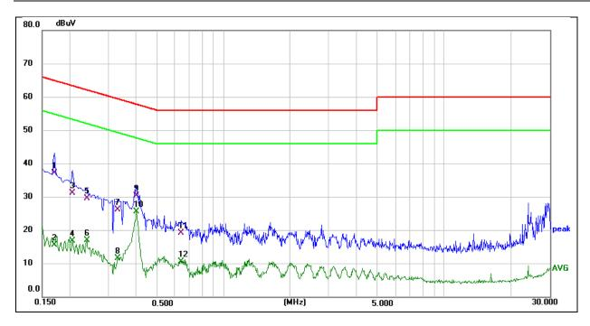
EUT: SmartSet Clock Radio Phase: N M/N.: ER100301 Temperature: 24
