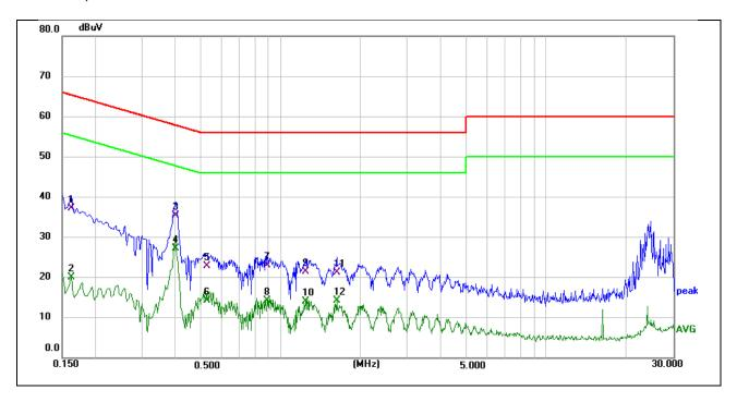
EUT: SmartSet Clock Radio Phase: **L1** M/N.: ER100301 **Temperature:** 24.3℃ Mode: 3-DH5 2480MHz **Humidity:** 52.6% RH **Test Engineer: Power Rating:** AC120V/60Hz Zero
