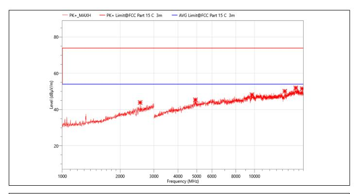
**EUT:** SmartSet Clock Radio **Temperature:** 24.5℃ M/N.: ER100301 **Humidity:** 55%RH **Power Rating:** Mode: 3-DH5 2441MHz AC 120V/60Hz **Test Engineer: Test Time:** 2023-08-03 **Berny**
