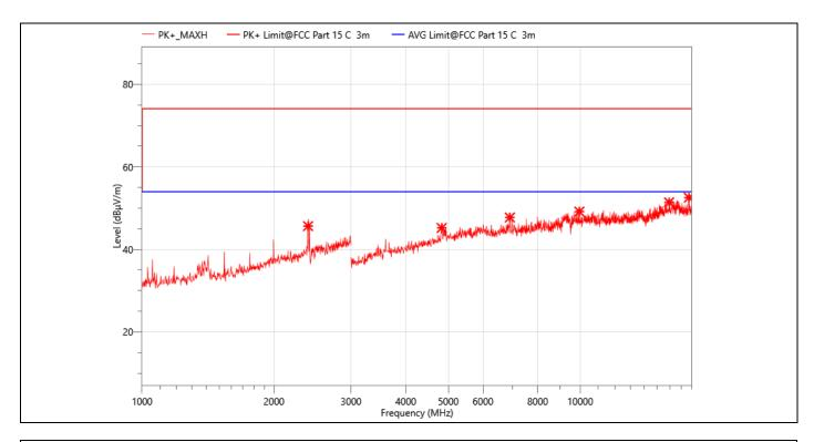
**EUT: SmartSet Clock Radio Temperature:** 24.5℃ M/N.: ER100301 **Humidity:** 55%RH Mode: 3-DH5 2480MHz **Power Rating:** AC 120V/60Hz **Test Engineer: Test Time:** 2023-08-03 **Berny**
