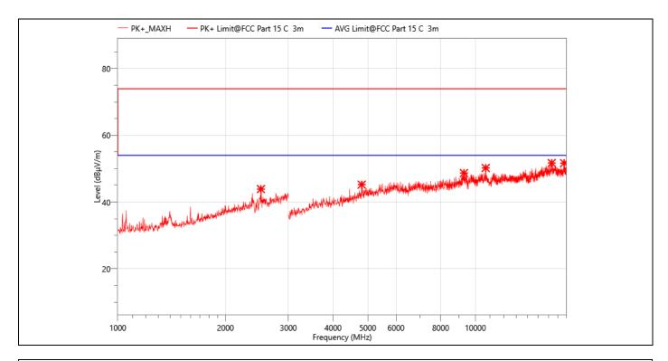
Temperature: **EUT:** SmartSet Clock Radio 24.5℃ M/N.: ER100301 **Humidity:** 55%RH **Power Rating:** Mode: 3-DH5 2480MHz AC 120V/60Hz **Test Engineer: Test Time:** 2023-08-03 **Berny**
