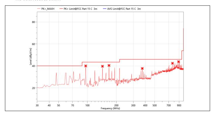
EUT: **SmartSet Clock Radio** Temperature: 24.5℃ M/N.: ER100301 **Humidity:** 55%RH Mode: 3-DH5 2480MHz **Power Rating:** AC 120V/60Hz **Test Time: Test Engineer:** Berny 2023-08-03
