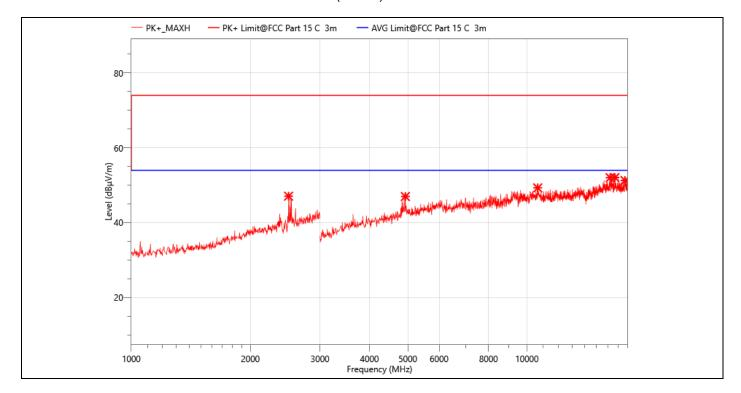
**EUT:** SmartSet Clock Radio Temperature: 24.5℃ M/N.: ER100301 **Humidity:** 55%RH Mode: 3-DH5 2402MHz **Power Rating:** AC 120V/60Hz **Test Engineer: Test Time: Berny** 2023-08-03
