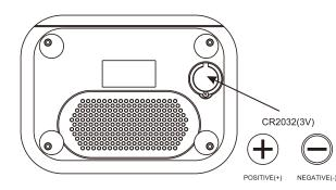
The lithium backup battery needs replacement when the LOW BATTERY indicator flashes, otherwise, the time and alarm settings will be lost/reset after a power outage
