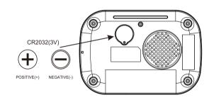
The lithium backup battery needs replacement when the LOW BATTERY ndicator flashes, otherwise, the time and alarm settings will be lost/rese after a power outage.
