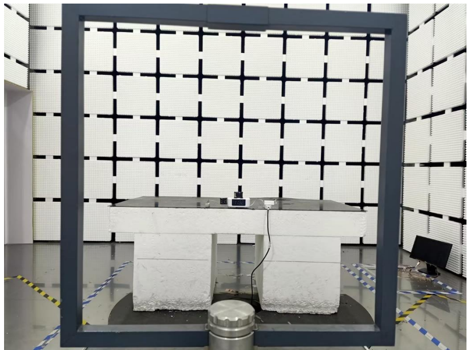
Radiation Emission Test Setup (Below 30MHz)
