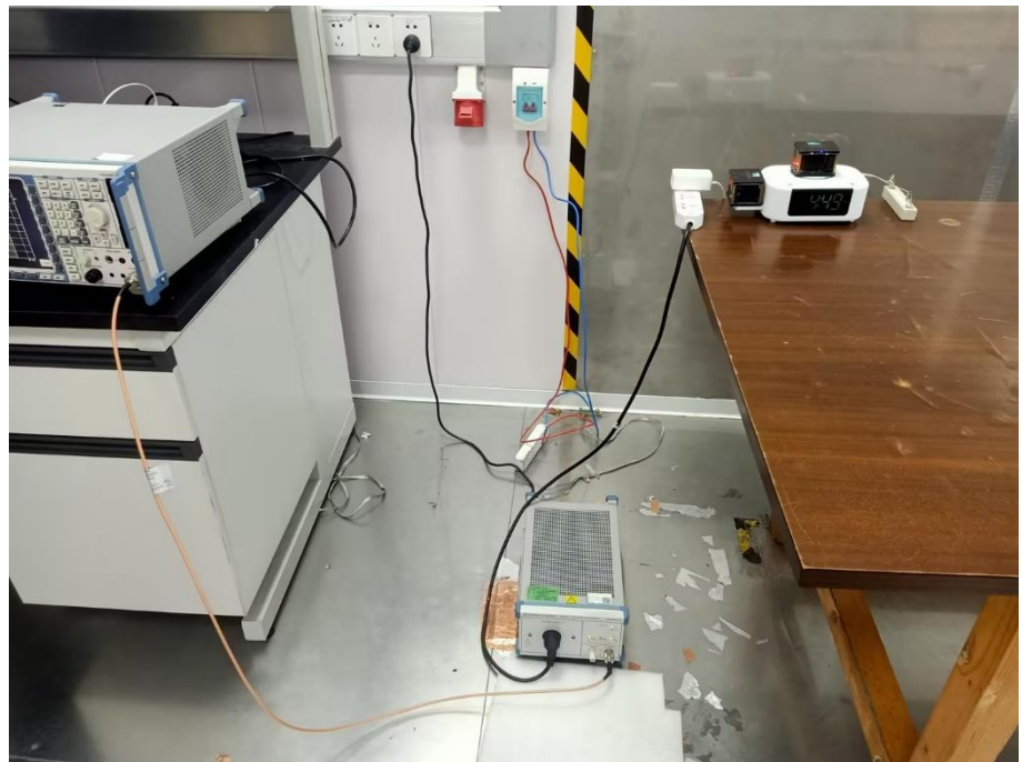
Conducted Emission Test Setup
