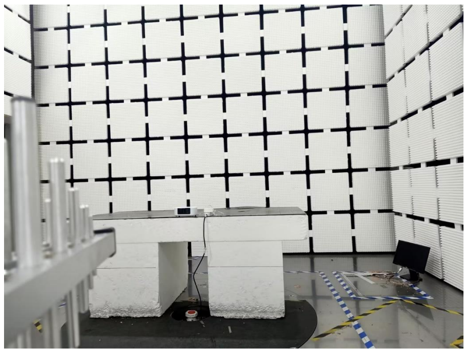
Radiation Emission Test Setup (30MHz to 1GHz)
