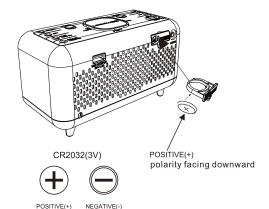
The lithium backup battery needs replacement when the LOW BATTERY indicator flashes, otherwise, the time and alarm settings will be lost/reset after a power outage.
