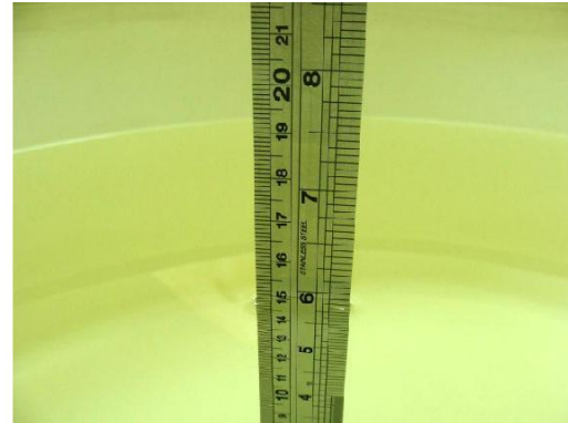
Fig 6.12 Photo of Liquid Height for Body SAR
