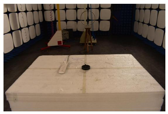
3. Radiated emission (9KHz-30MHz)
