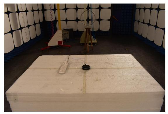
3. Radiated emission (9KHz-30MHz)
