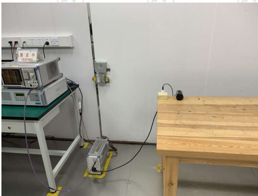
AC Power Line Conducted Emission
