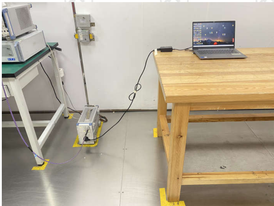
Conducted Emissions Test Setup-1
