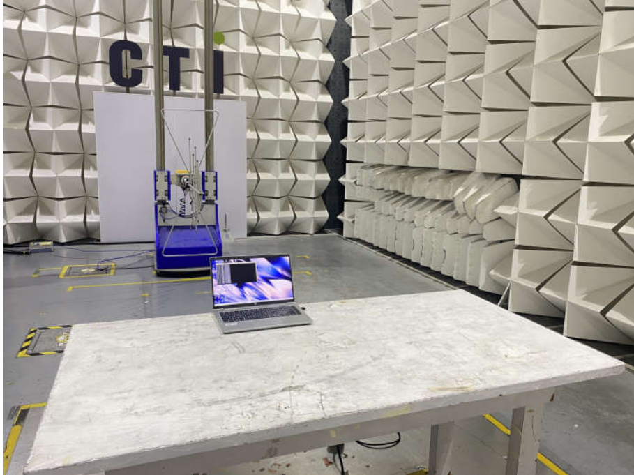
Radiated spurious emission Test Setup-1(Below 1GHz)
