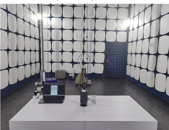
3. Radiated emission (9KHz-30MHz)
