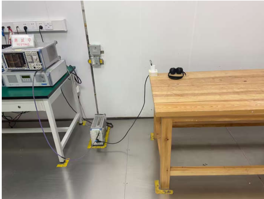
Conducted Emissions Test Setup
