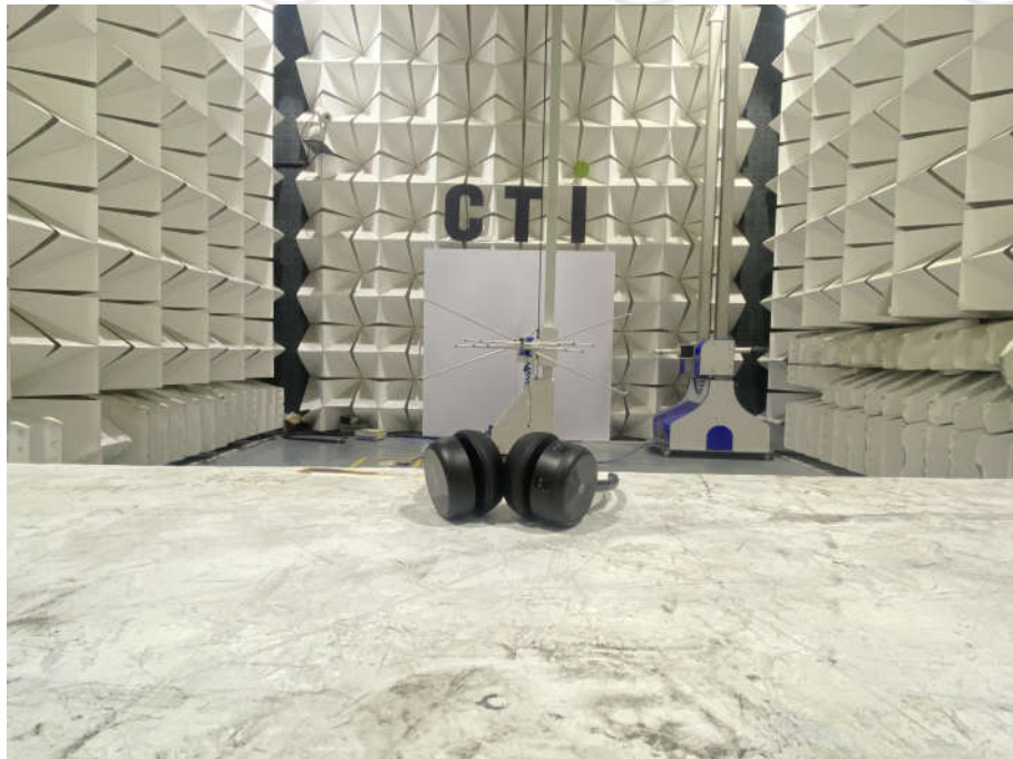
Radiated spurious emission Test Setup-2(Below 1GHz Close up)
