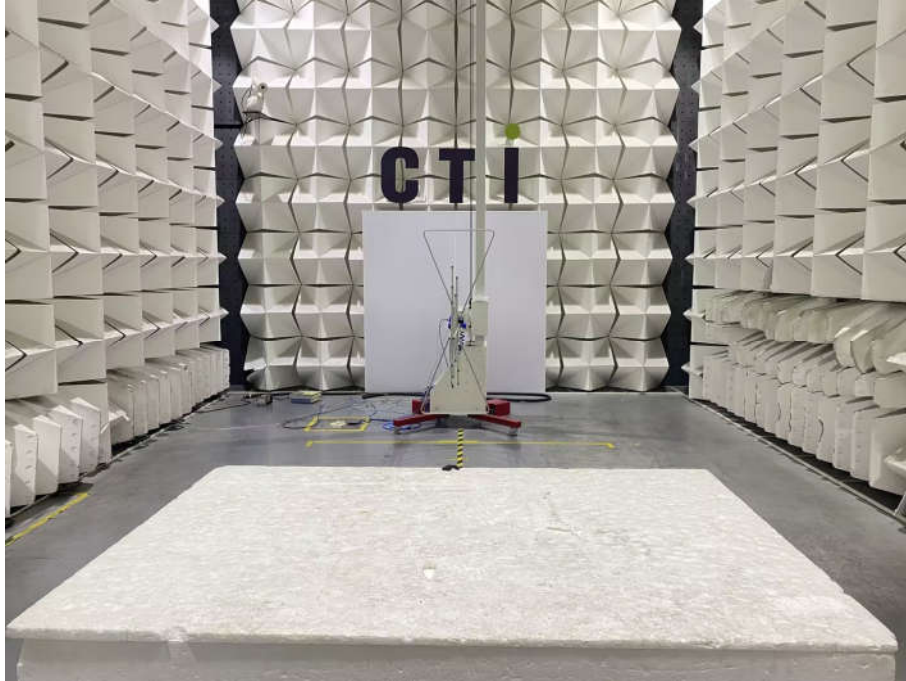
Radiated spurious emission Test Setup-1 Left ear (Below 1GHz)
