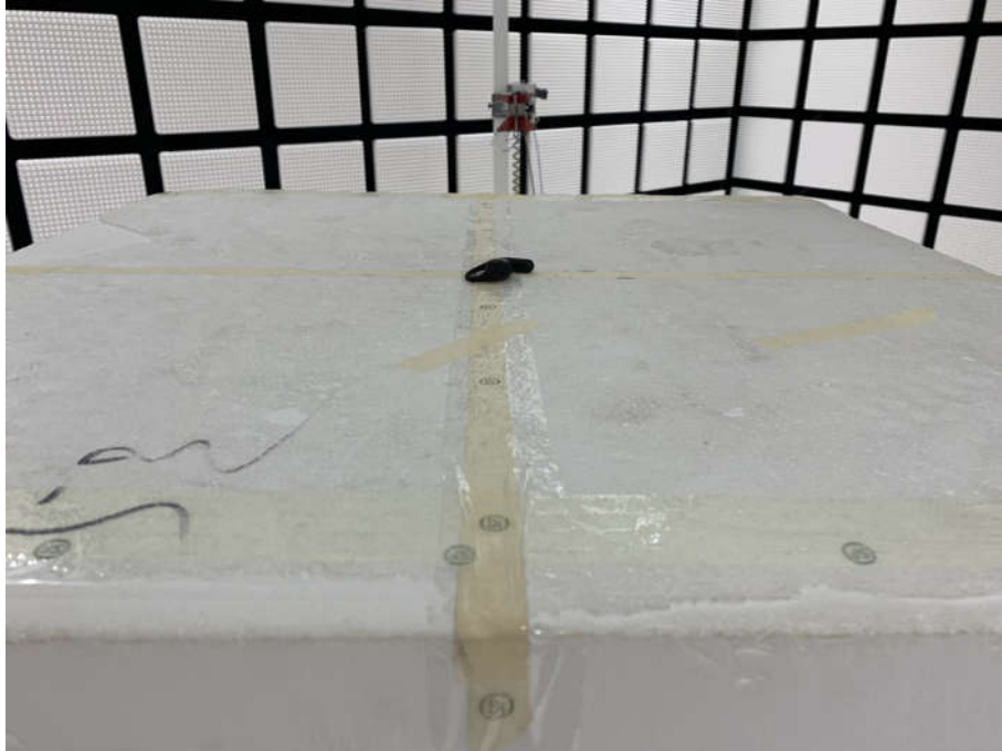
Radiated spurious emission Test Setup-3 Left ear(Above 1GHz)
