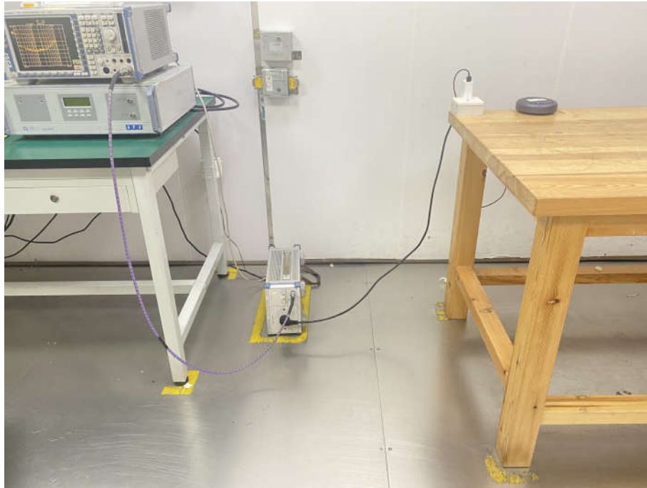
Conducted Emissions Test Setup-1
