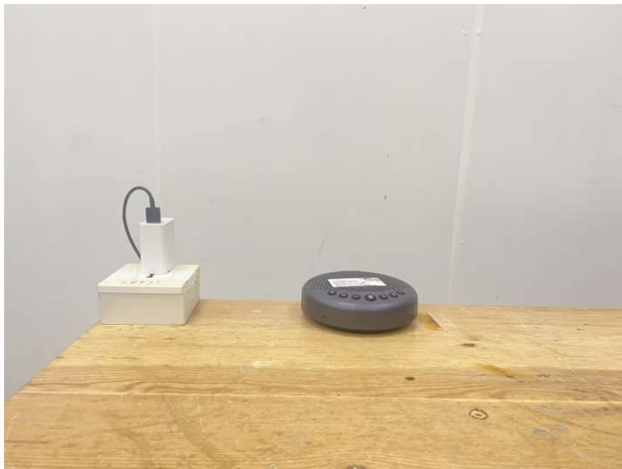
Conducted Emissions Test Setup Close up-2
