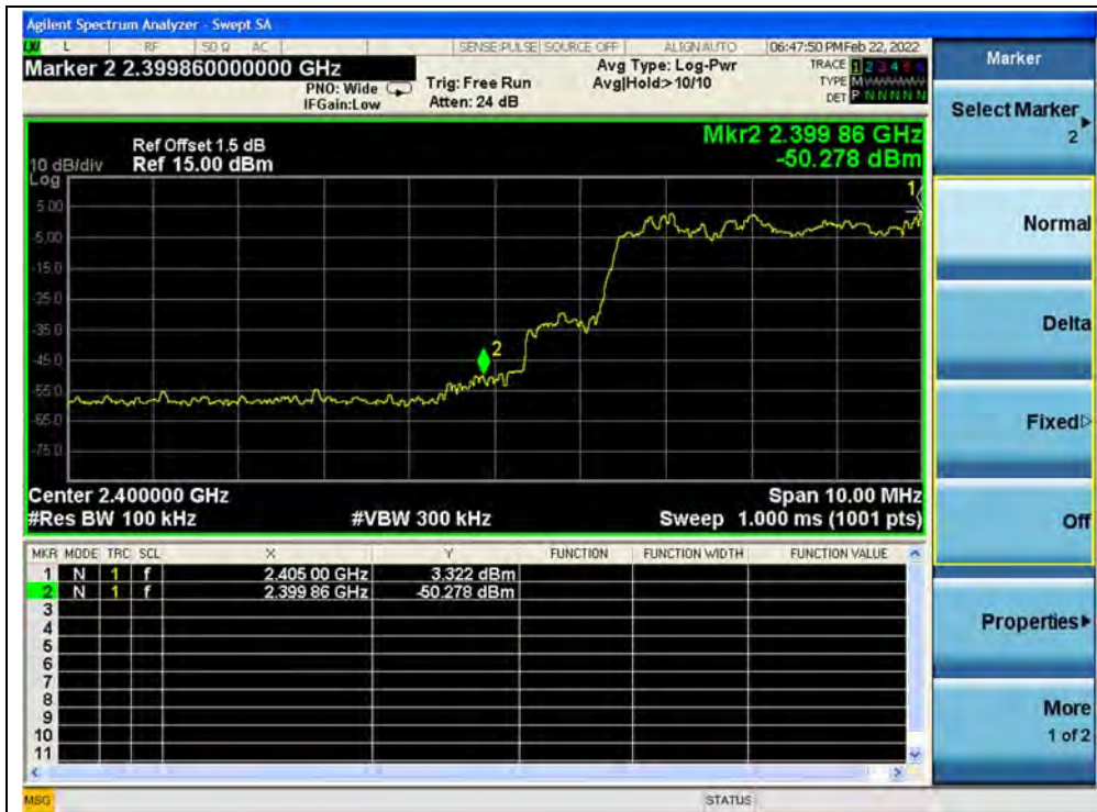
(Band edge with hopping on, Channel 0, 8-DPSK)
