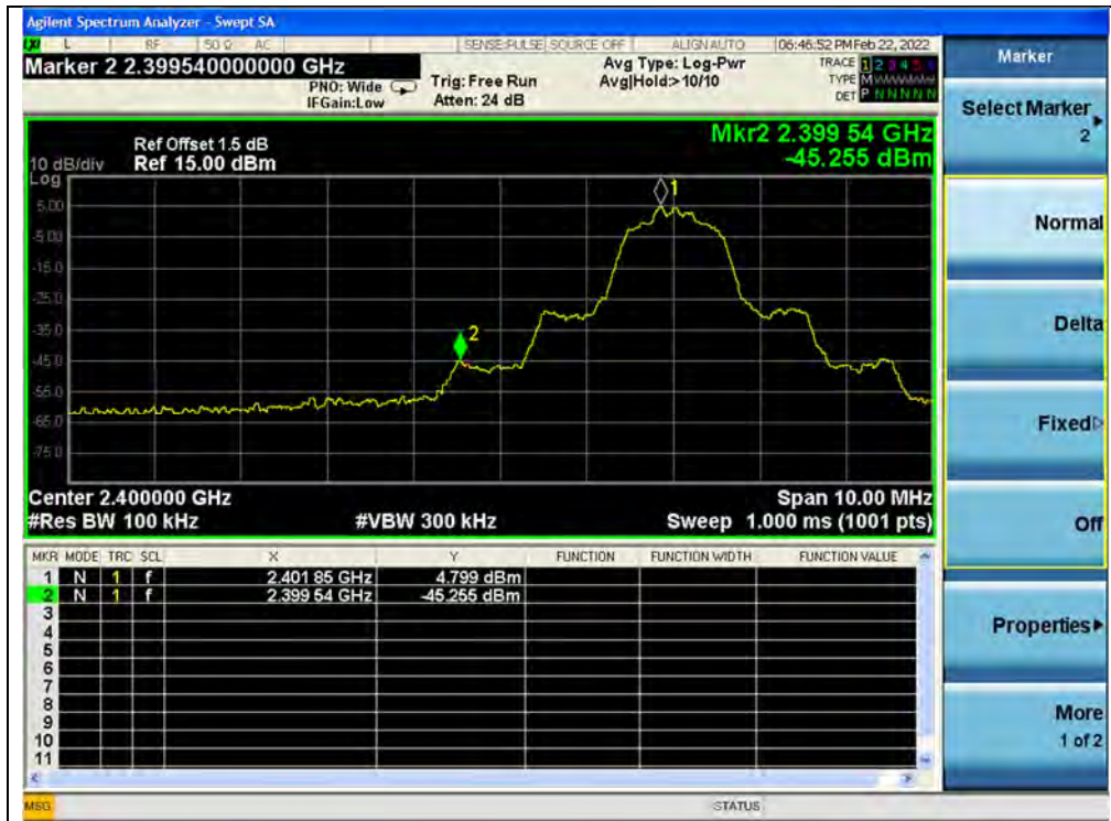
(Band edge, Channel 0, \pi/4 -DQPSK)
