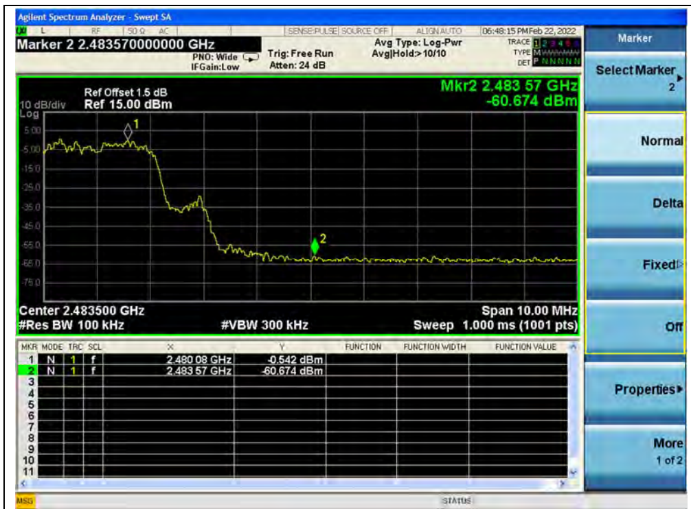
(Band edge with hopping on, Channel 78, 8-DPSK)
