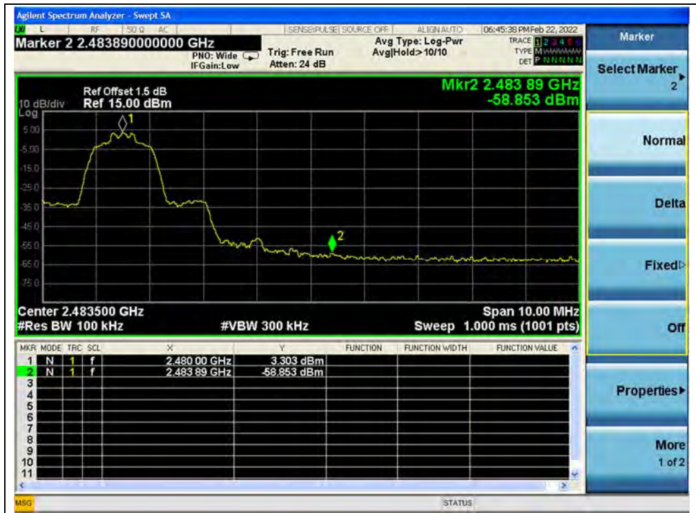
(Band edge, Channel 78, \pi/4 -DQPSK)
