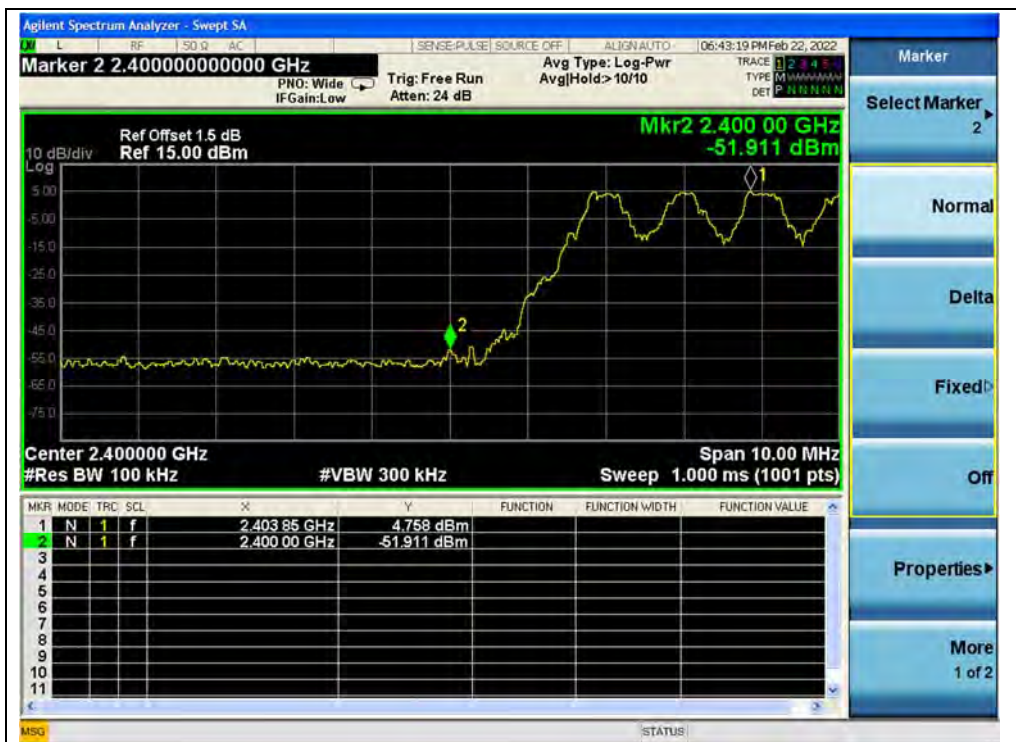
(Band edge with hopping on, Channel 0, GFSK)
