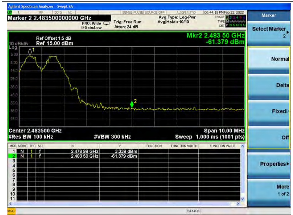
(Band edge with hopping on, Channel 78, GFSK)
