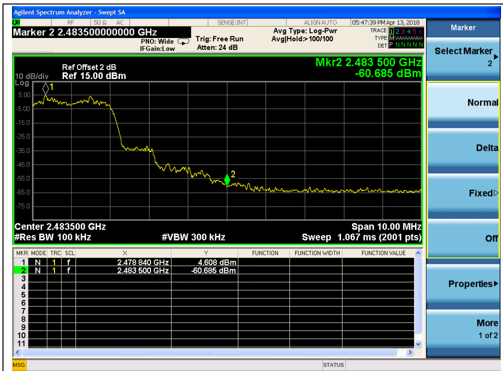
(Channel = 78, Band edge with hopping on, 8-DPSK)
