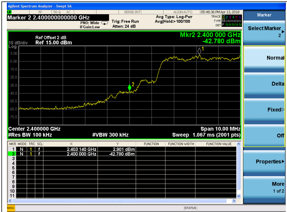
(Channel = 0, Band edge with hopping on, 8-DPSK)
