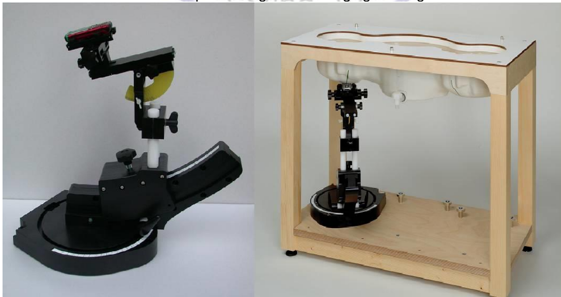
Device holder supplied by SPEAG
