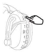
2. Press and hold the Power/Mode button for three seconds to turn the headphones On
