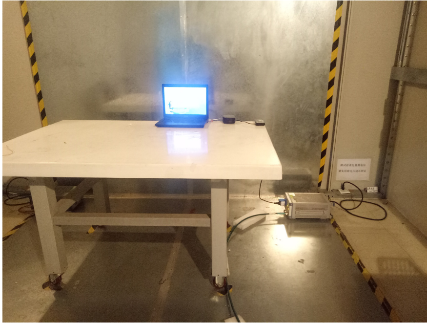
Conducted Emissions (Side View)
