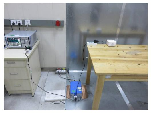
FCC RADIATED EMISSION TEST SETUP
