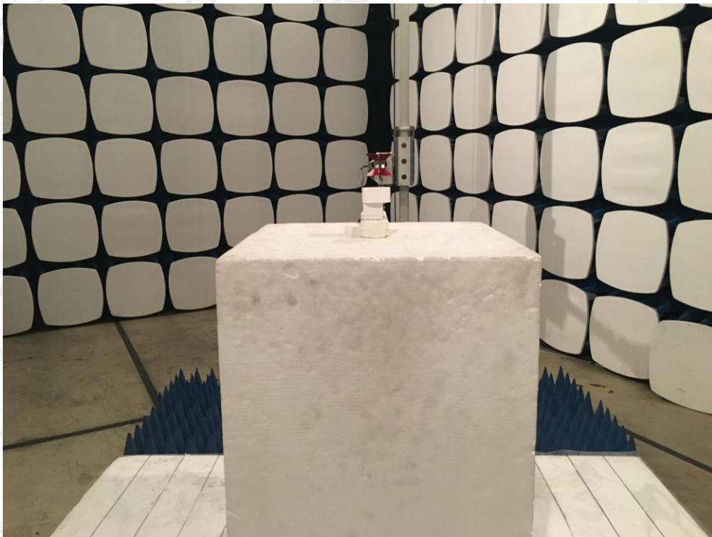
FCC RADIATED EMISSION TEST SETUP ABOVE 1GHZ
